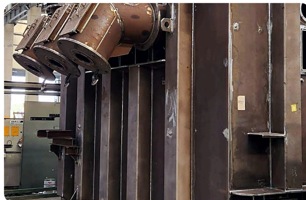
Power transformer tank in fabrication
